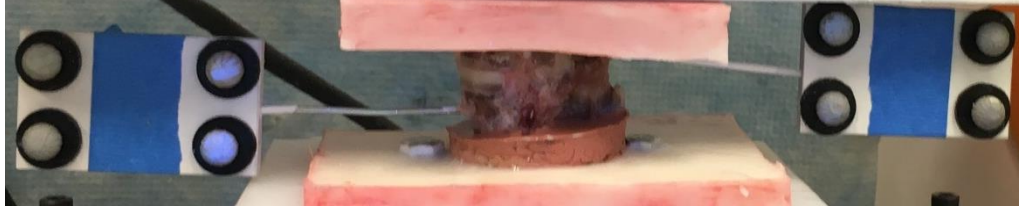
Figure 18: Reflective Marker Orientation and Attachment to Each Vertebra.
