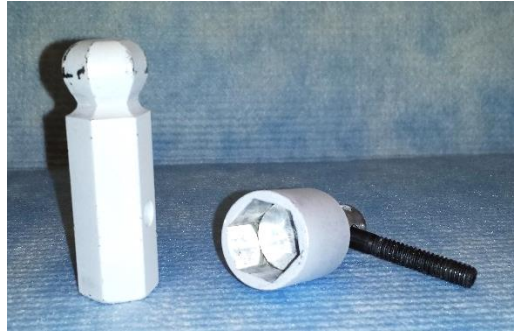
Figure 14: Hex Joint. Used to apply pure moments in axial rotation.
